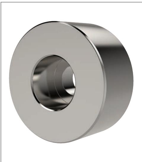
Pads of 17-4 Stainless, hardened to RC 43/46 provide solutions to applications where material selection is of greater importance; for example nuclear or food processing or pharmaceutical applications.
